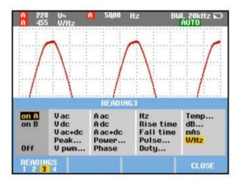
Figure 3. Selecting the V/Hz ratio for measurements carried out on input A.
