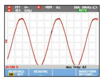
Figure 4. Measuring Vpwm and Hz, and displaying the V/Hz ratio.
