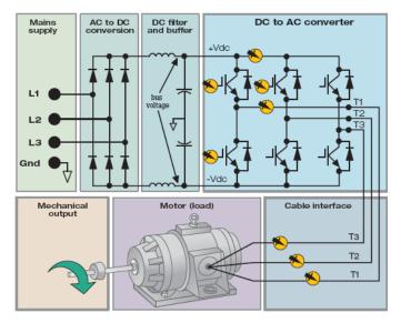
Figure 1. Basic electric schematics of variable-speed drive.
